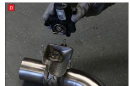
A) After you have removed O.E exhaust you will need to remove the rear valve motor (left hand side). remove 3 x 8mm nuts ( keep safe as you will need them to bolt the electronic valve motor to Scorpion Exhaust).
